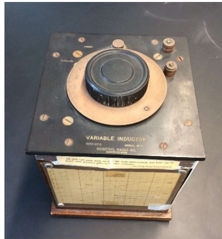
Figure 9: Type 107 Variable Inductor, circa 1918-1927
